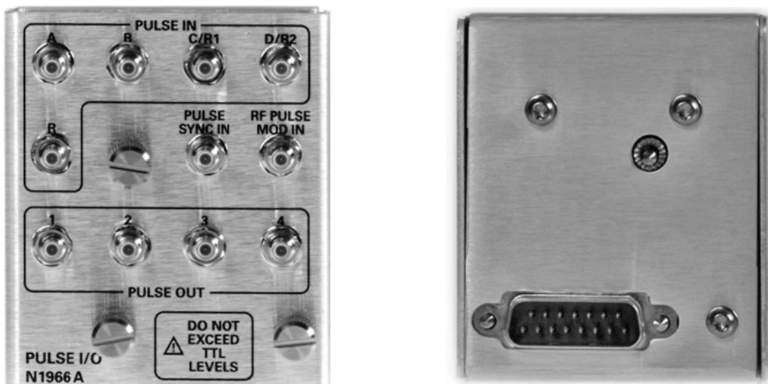
Figure 2-1 N1966A Pulse I/O Adapter
